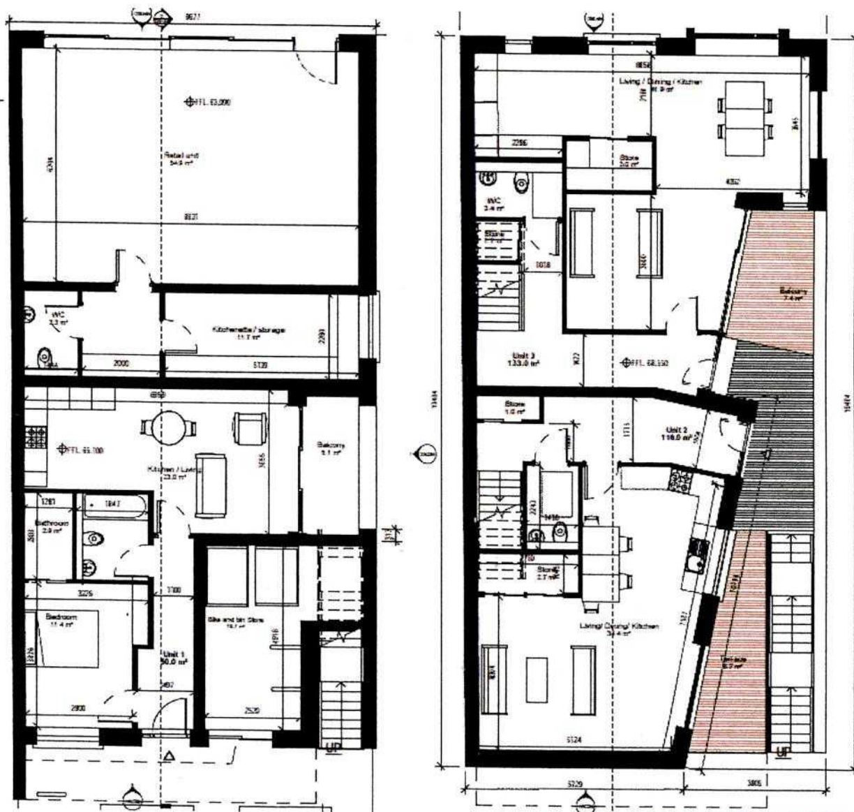
Figure 3.0 Ground (left) and first (right) floor plans proposed development (as per alternative design option B).
