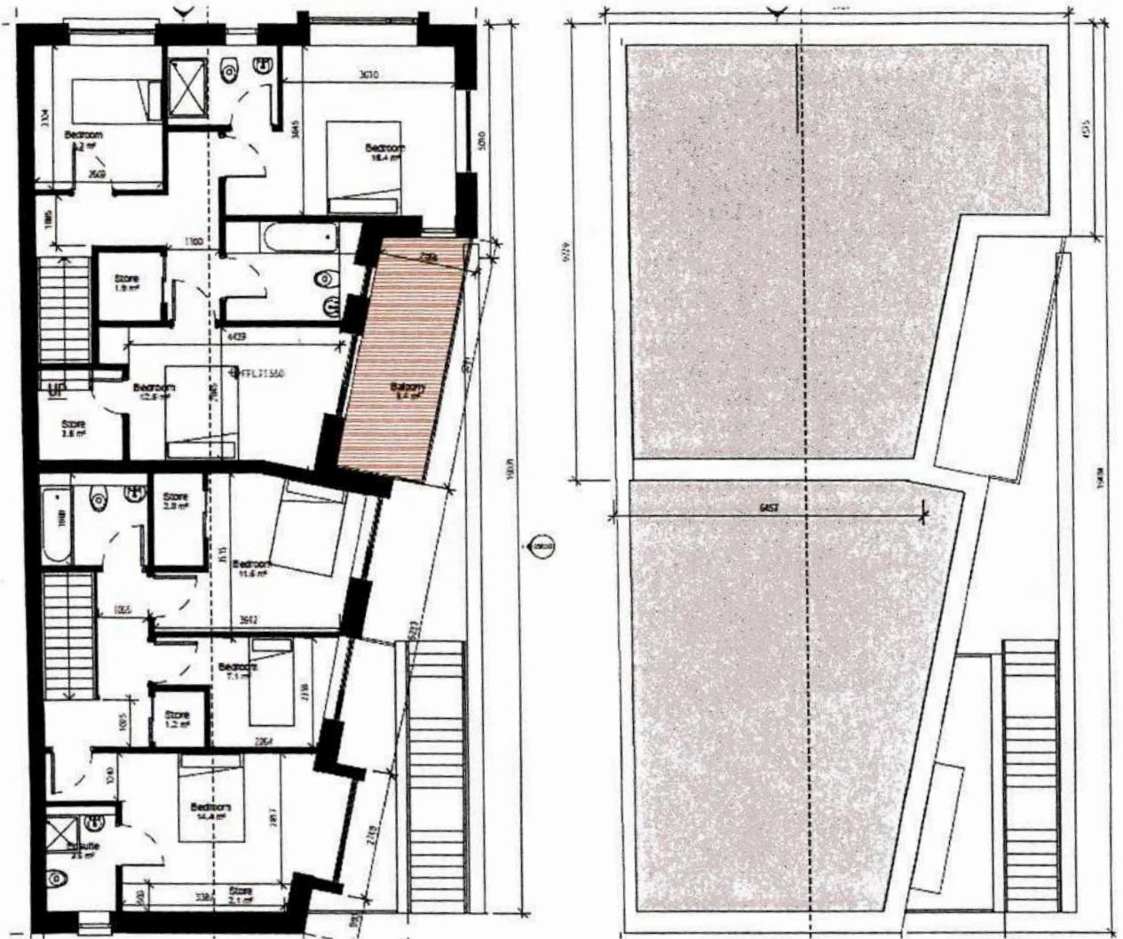
Figure 4.0 Second (left) and roof (right) floor plans proposed development (as per alternative design option B).
